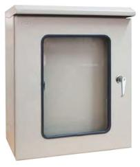
Wall-Mount Outdoor Fiber made of sheet EG Steel or stainless steel or Aluminium make to order one by one They can compliant with IP55 standard. they can accommodate the fiber optic solution, CCTV, Broadband Cable entry 3 port use cable glands EG/PG29 depand on cable dia. The cable can be held the preformed holes, inside a 2 section cable inlet or cable feed through gromment.
